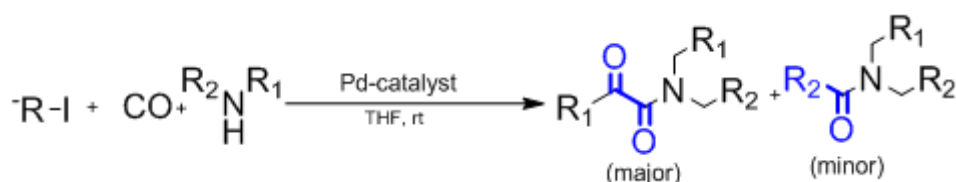
Scheme 8. The first catalytic approach to alpha-ketoamides by amino double carbonylation.
